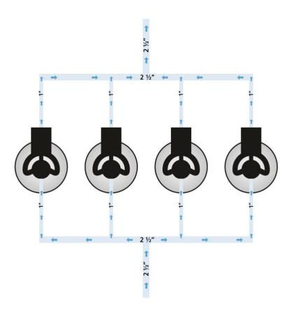
The blue arrows represent the water flow. The plumber/installer will build a manifold with four 1-inch outlets that connect to the water filters. The process will be repeated on the other side, connecting the manifold to the pipe that delivers water to the building. The exact placement of the units will vary depending on the installation area.
